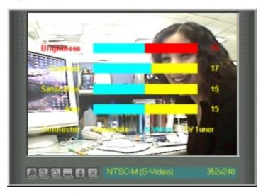
Use your mouse/pointing device or the UP and DOWN arrow keys on your keyboard to select options (*Brightness, Contrast, Saturation, Hue, Connector*) and then the LEFT (select to the left or to decrease) or RIGHT (select to the right or to increase) arrow keys to change an option. You may also use your mouse/pointing device to change an option by clicking the appropriate item or slider.
